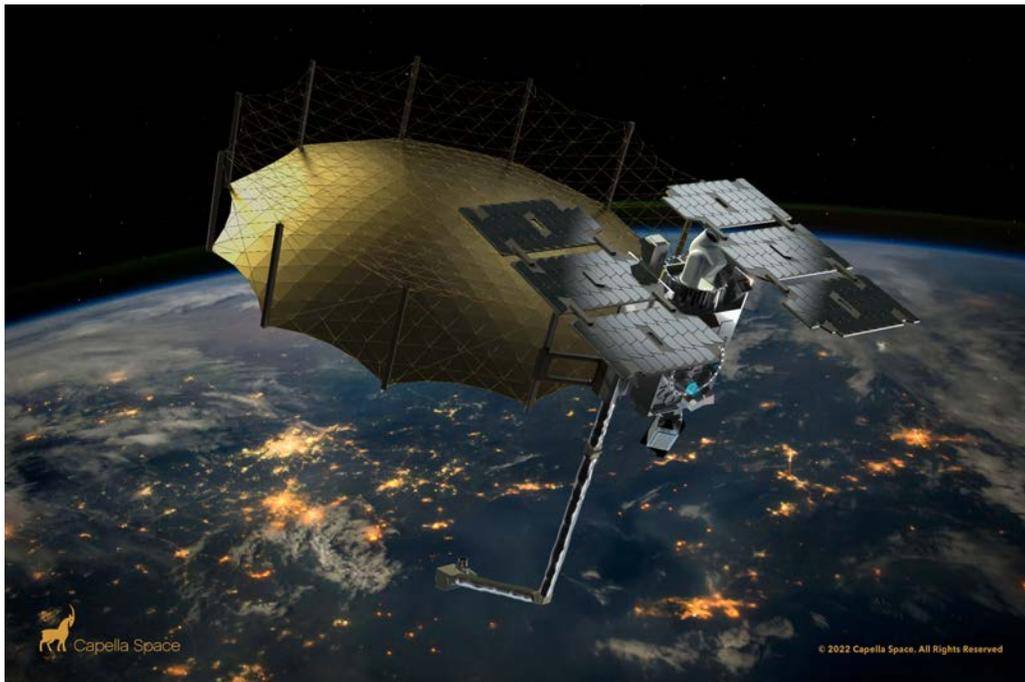
Figure 55. Capella’s next generation Acadia synthetic aperture radar (SAR) satellite with 21 cm (slant range) to 31 cm (ground range) resolution and optical inter-satellite links that are compatible with the Space Development Agency’s National Defense Space Architecture. (Credit: Capella Space)<sup>322</sup>
