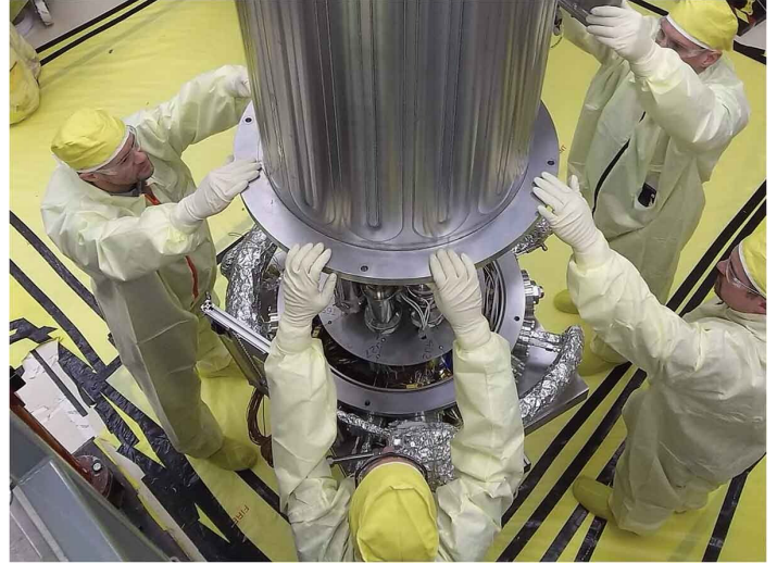
Photo 1: Computational simulation of the Antares RI microreactor core, highlighting the prismatic graphite blocks and reactivity control drums. [Credit: Antares]; Photo 2: NASA and NNSA engineers lower the vacuum chamber wall around the Kilowatt Reactor Using Stirling Technology (KRUSTY) to simulate space conditions. [Credit: Los Alamos National Laboratory]
